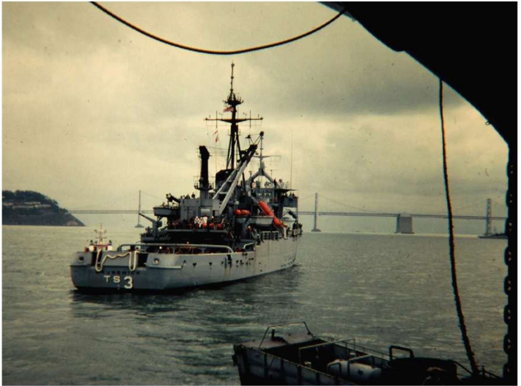
Easing the xUSS Oriskany CVA-34 towards the stern of the USS Brunswick ATS-3 with a “pusher-boat” from Port Services Treasure Island to run out a messenger attached to the xUSS Oriskany CVA-34’s anchor chain to the USS Brunswick ATS-3 for connection to the nylon towing hawser.
