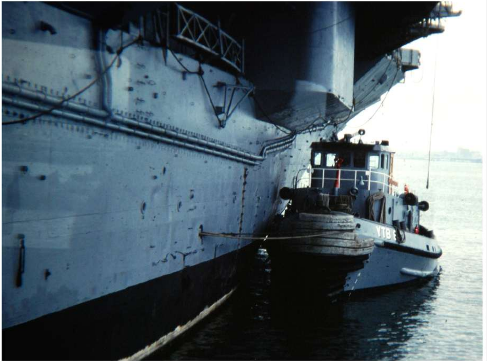
N/V Accomac YTB-812 made-up power to the port quarter of the xUSS Oriskany CVA-34.
