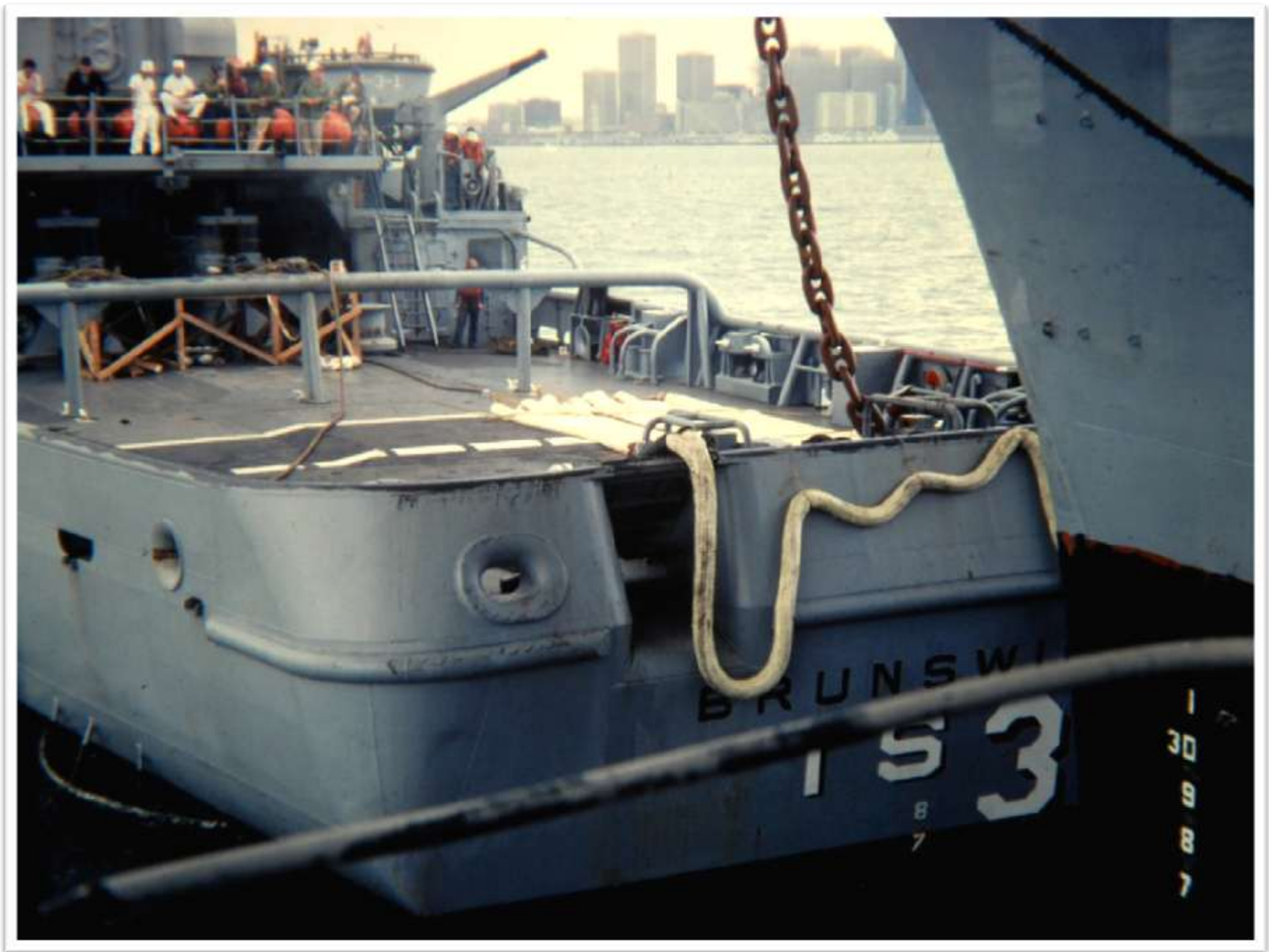
“Close enough for you?” Crew of the USS Brunswick ATS-3 hooking up the nylon towing hawser. The nylon towing hawser was special ordered from Samson Ocean Systems and was 1,200 feet long, 14” in circumference with encapsulated eyes which included the then new Nylite Rope Connectors.
