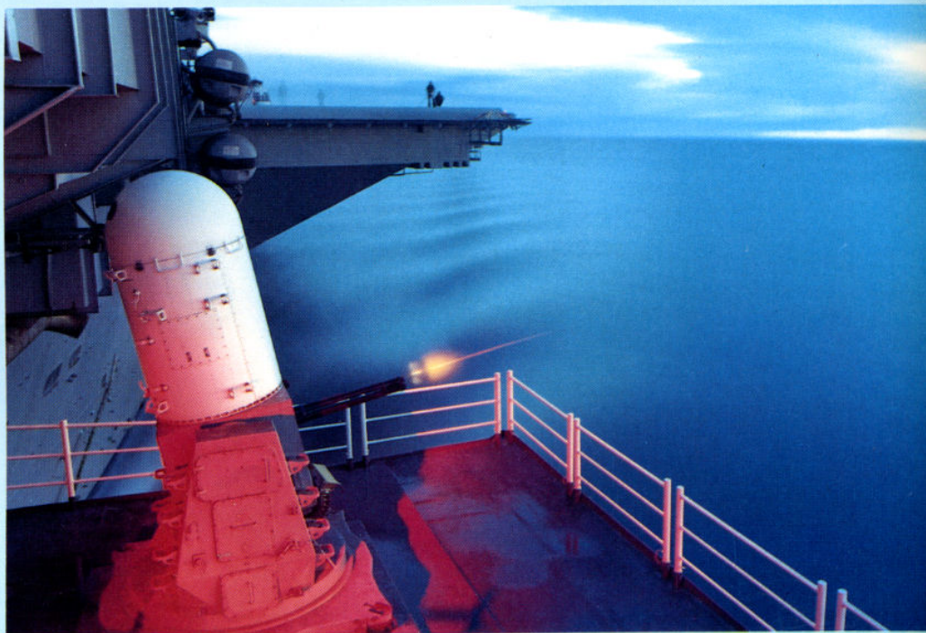
One of three Close In Weapons Systems (CIWS) on board, the CIWS is capable of firing 3,000 rounds per minute to protect the ship from hostile aircraft.
