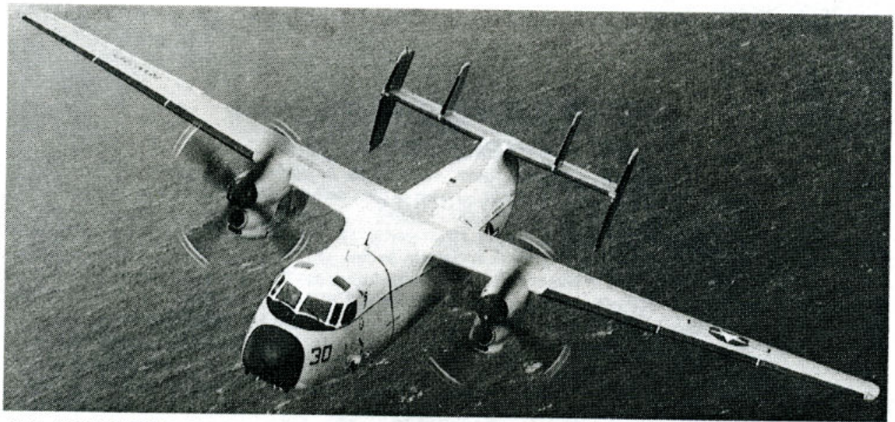
C-2A GREYHOUND: The C-2A Greyhound is the "Carrier On board Delivery" (COD) aircraft. The C-2A provides a means to transport spare parts, mail and people to and from the ship. A two-plane detachment from the VRC-30 "Providers" flies in CVW-2.
