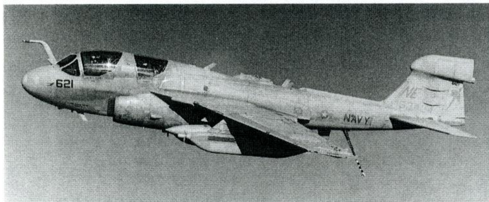
EA-6B PROWLER: A four-seat electronic countermeasures aircraft, the VAQ-131 "Lancers" fly the ICAP-2 version of the Prowler. An improved jamming capacity, expanded communications system, enhanced signal processing and the HARM missile make the EA-6B the platform of choice for suppression of enemy air defense systems and protection of CVW-2 strike aircraft as they put ordnance on target and safely egress.
