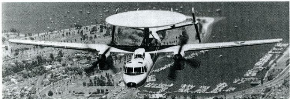
E-2C+ HAWKEYE: The "eyes" of CVW-2, this airborne early warning command and control aircraft keeps the big picture for the battle group. The VAW-116 "Sun Kings" fly the updated version of the Hawkeye. This E-2C+, with a crew of five, operates at longer ranges, can track over 2000 targets, has improved jamming resistance and fully-automated/optimized overland detection. State-of-the-art avionics and upgraded engines make this "mini-AWACS" an indispensable command and control platform.
