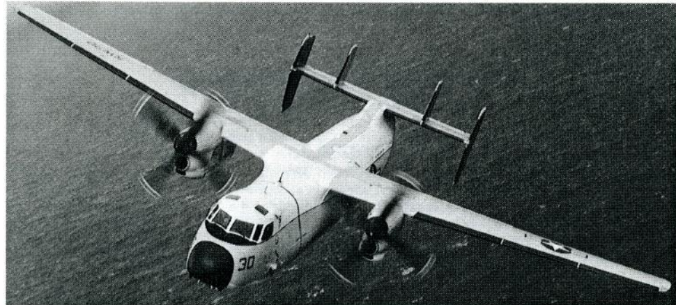
C-2A GREYHOUND: The C-2A Greyhound is the "Carrier On board Delivery" (COD) aircraft. The C-2A provides a means to transport spare parts, mail and people to and from the ship. A two-plane detachment from the VRC-30 "Providers" flies in CVW-2.
