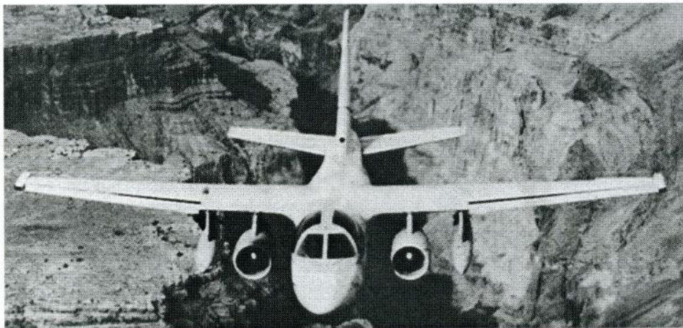
S-3B VIKING: A four-seat extended-range force multiplier, this aircraft is the "long pole in the tent" for CVW-2. While incorporating an improved anti-submarine weapons system, this upgraded Viking has evolved into a platform relied upon to perform multiple missions. Equipped with an imaging radar, improved avionics, the Harpoon missile, and an in-flight refueling system, the S-3B provides unique offensive punch and support to the battle group. The VS-38 "Red Griffins" fly in CVW-2.
