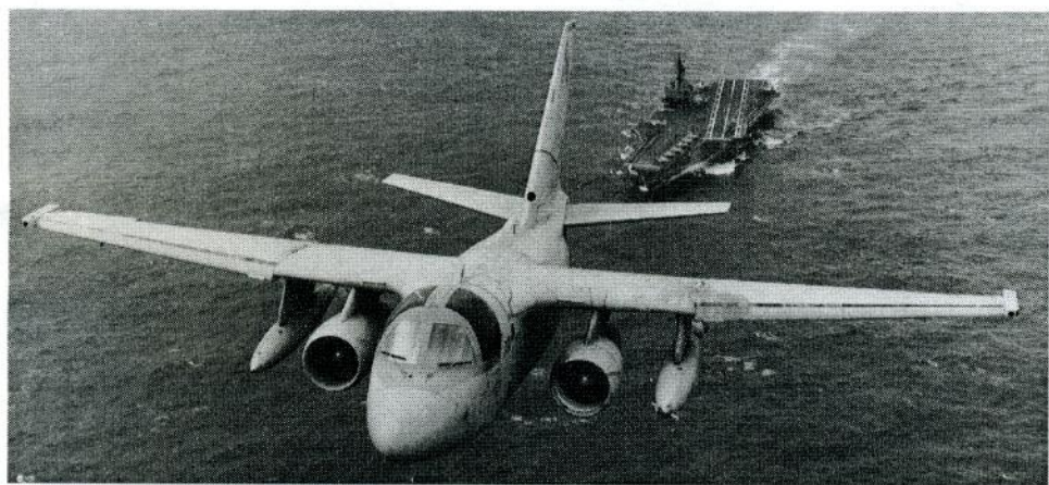
ES-3A SHADOW: CVW-2 incorporates a two-plane detachment of ES-3A electronic reconnaissance aircraft. This variant of the S-3A provides the battle group its own sensor suite to scout and exploit the electronic emissions of adversary forces at extended ranges. While retaining airframe commonality with the S-3A, the ES-3A has entirely new avionics and signal processing capabilities. The VQ-5 Det Delta "Sea Shadows" fly in CVW-2.
