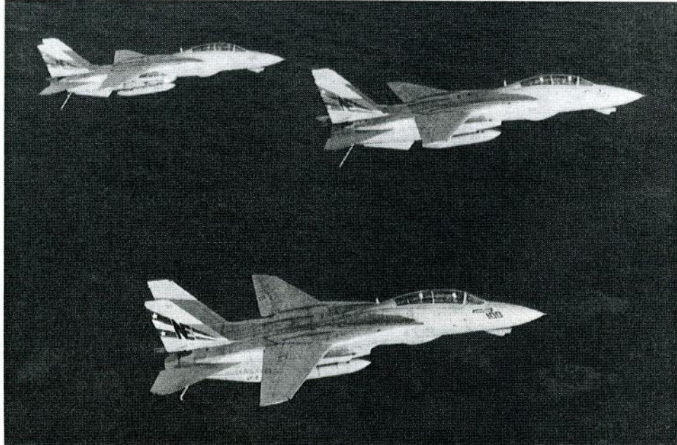
F-14D SUPER TOMCAT: A two-seat, long-range, supersonic interceptor with attack capability. Outfitted with new engines, the F-14D enjoys increased fuel efficiency and unrestricted throttle handling throughout its flight envelope, including catapult launches without the use of afterburners. Improved radar and enhanced missile capability give the star of "TOP GUN" a decisive edge in the air-to-air arena. The VF-2 "Bounty Hunters" are the sole F-14 Tomcat squadron in CVW-2.
