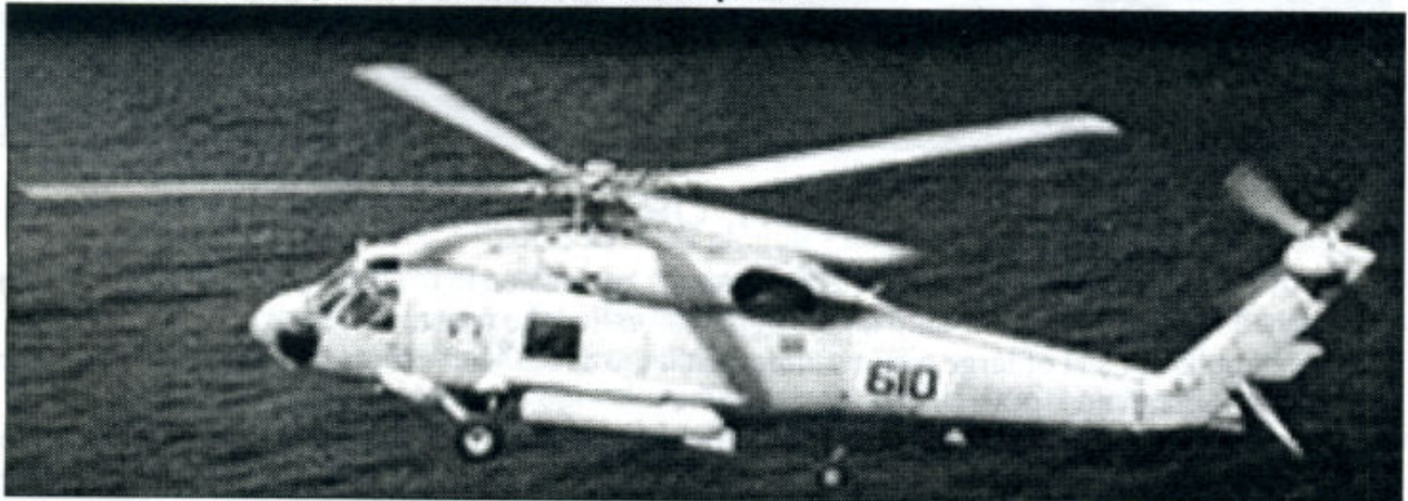
SH-60F / HH-60H SEAHAWK: Incorporating an integrated antisubmarine mission avionics system with a dipping sonar, a crew of four provides inner-zone protection for the carrier as well as primary Sea Air Rescue (SAR) responsibility. Other primary mission areas include strike rescue and special warfare support. The HS-2 “World Famous Golden Falcons” complete the total combat package for the air wing.
