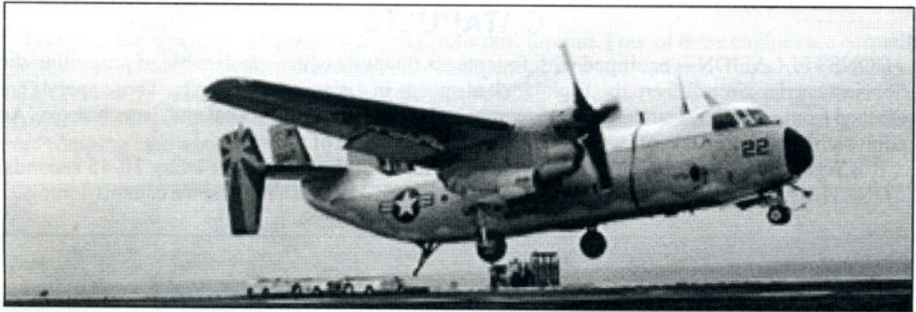
C-2A GREYHOUND: The C-2A Greyhound, also known as the “Carrier On board Delivery” (COD) aircraft, provides critical logistics support. With a payload of up to 10,000 pounds, the C-2A provides a means to transport spare parts, mail and people to and from the ship. A two-plane detachment from the VRC-30 “Providers” flies in CVW-2.
