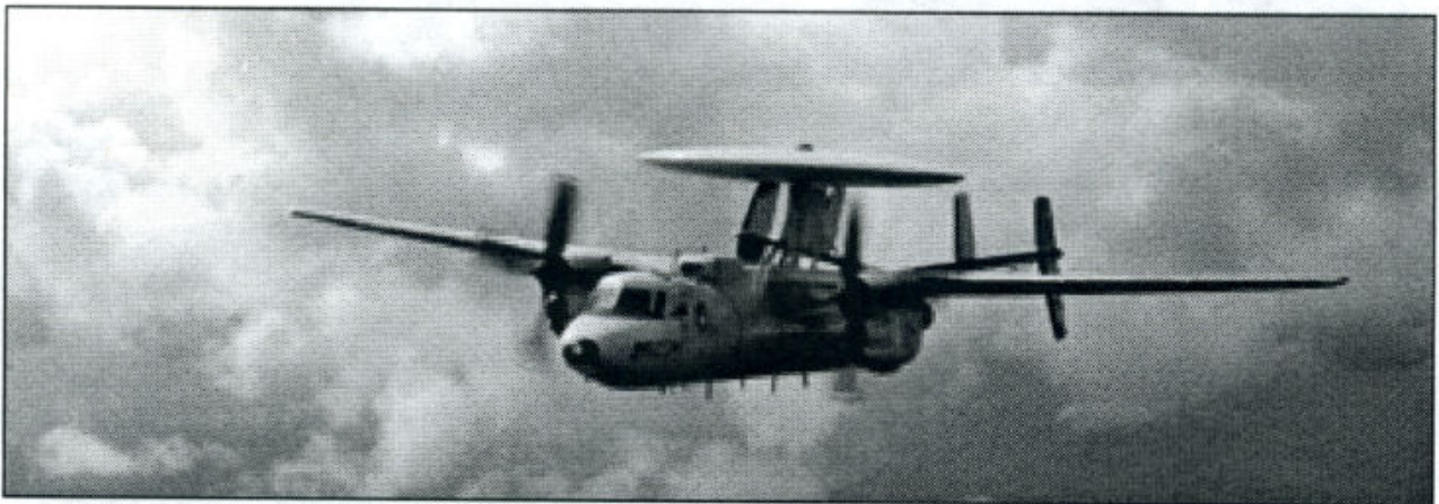
E-2C+ HAWKEYE: The “eyes” of CVW-2, this airborne early warning command and control aircraft keeps the big picture for the battle group. The VAW-116 “Sun Kings” fly the updated version of the Hawkeye. This E-2C+, with a crew of five, operates at longer ranges, can track more than 2,000 targets, has improved jamming resistance and fully-automated/optimized overland detection. State-of-the-art avionics and upgraded engines make this “mini-AWACS” an indispensable command and control platform.
