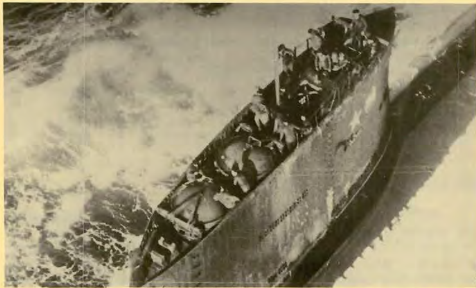
The two missile tubes of a Zulu V.
