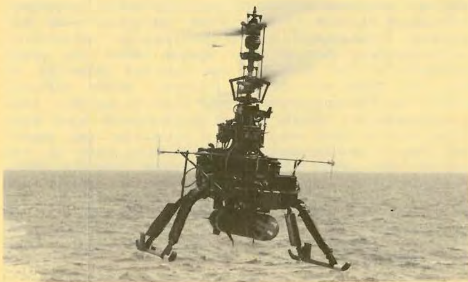
(A) An early DSN-1 DASH vehicle with a single homing torpedo hovering over Hazelwood's stern.
