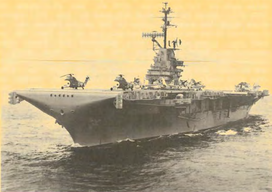
(B) USS Yorktown (CVS 10) with HSS-1 helicopters, S2Fs and AD-5W AEW aircraft. Note the angled deck, enclosed bow and reduced armament typical of the 27A-125 conversions.
