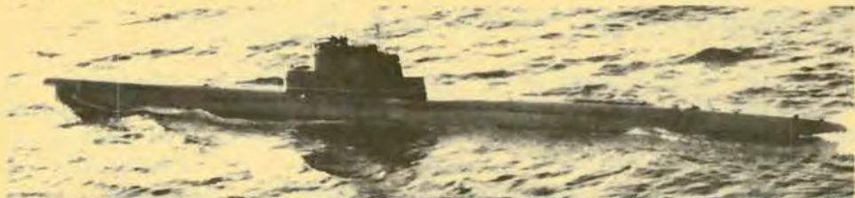
An early Whiskey II submarine in the North Atlantic. At some 235 units, this was the Soviets' most numerous postwar class.
