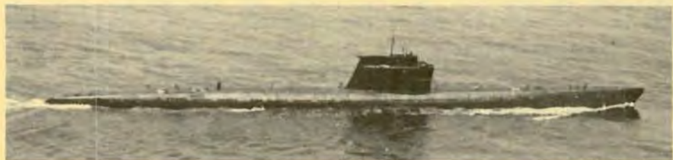
A Zulu III, a 2,500-ton design believed strongly influenced by the German Type XXI. Some thirty-two were built during the fifties.
