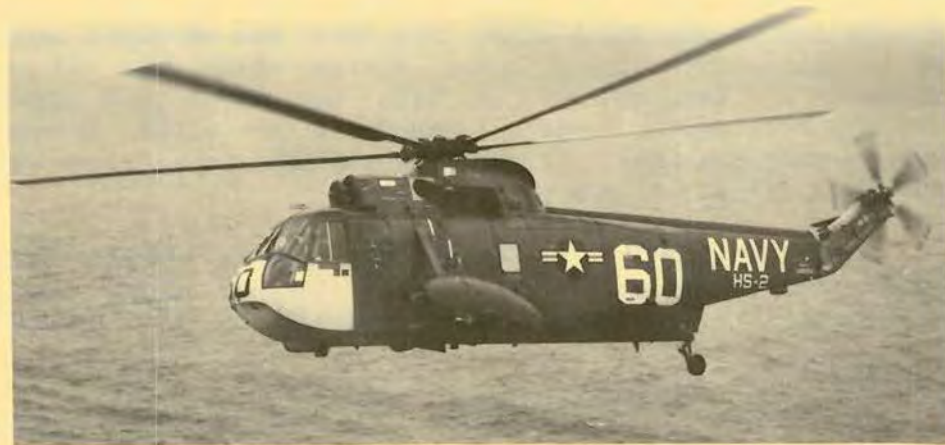
The HSS-2 (SH-3A) Sea King. First flight for this ASW helicopter of the sixties was 11 March 1959. It carried the much improved AQS-10 sonar.
