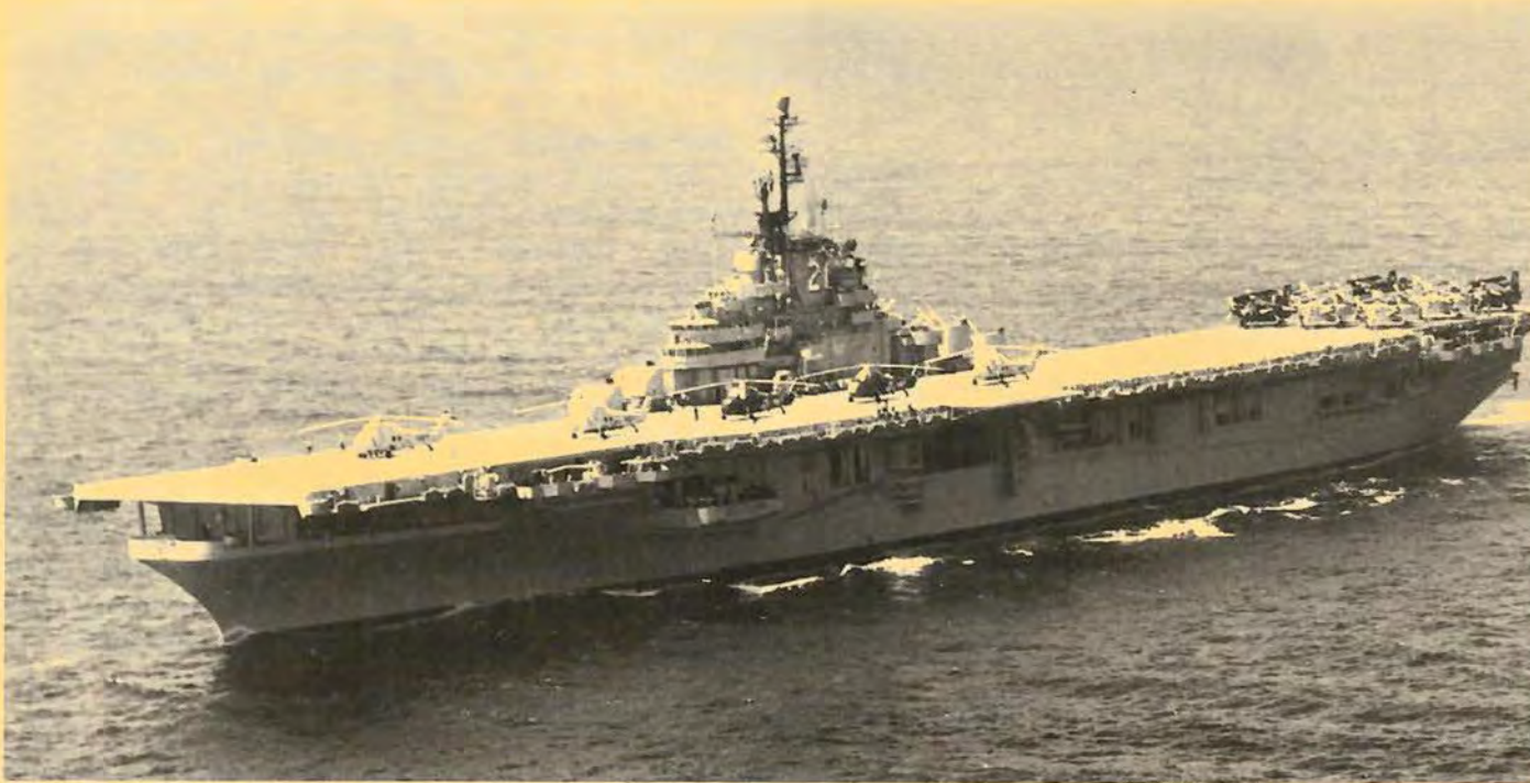
(A) Boxer (CVS 21) as a CVS. Note the early TACAN, the HSS-1 helicopters and S2F aircraft. May 1956.
