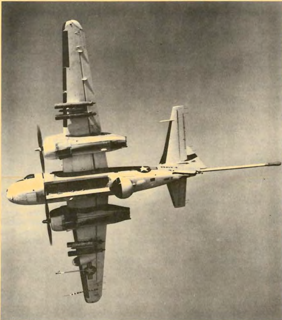
(B) An S2F-1 with everything: radar and MAD extended, searchlight, four Mk 43 torpedoes, two high velocity rockets and Lulu hidden in the bomb bay.
