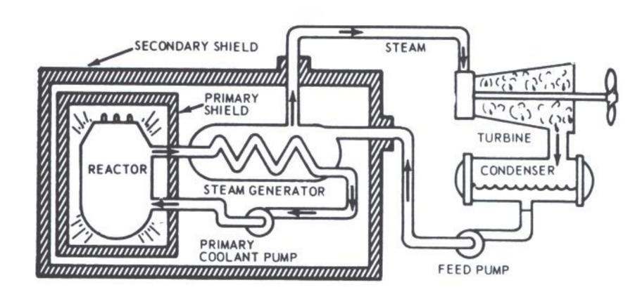
There is no step in the generation of this power which requires the presence of air or oxygen. This fact alone allows the ship to operate completely independent from the earth's atmosphere for extended periods of time.
