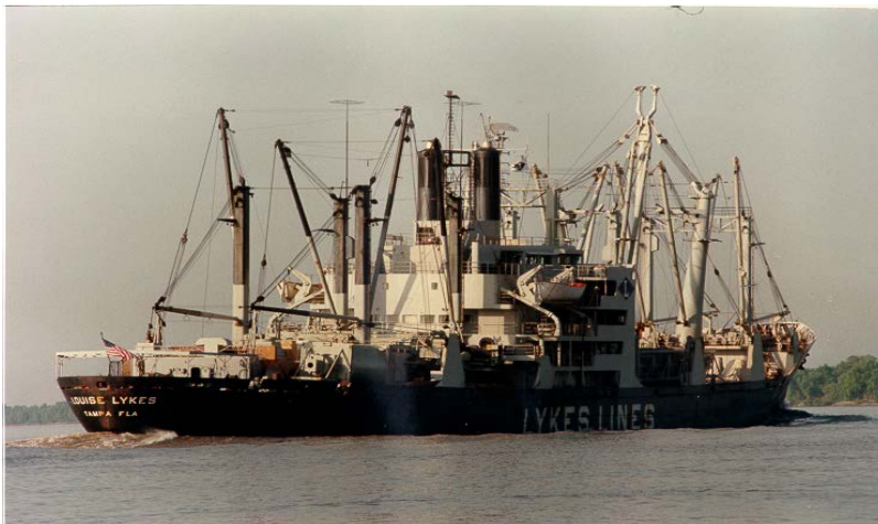
Bottom: Louise Lykes circa 1960s. Note the kingpost & booms with the heavy lift boom forward, raised forecastle and superstructure (with machinery below) at the 2/3 aft position. Maritime Administration photographs.
