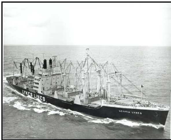
Top: Letitia Lykes underway circa 1968. Lykes Lines vessels of the C4-S-66a class display many of the common features of the general cargo break-bulk vessel.
