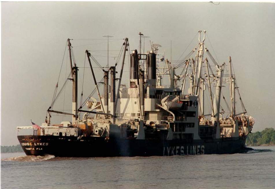
Bottom: Louise Lykes circa 1960s. Note the kingpost & booms with the heavy lift boom forward, raised forecastle and superstructure (with machinery below) at the 2/3 aft position. Maritime Administration photographs.
