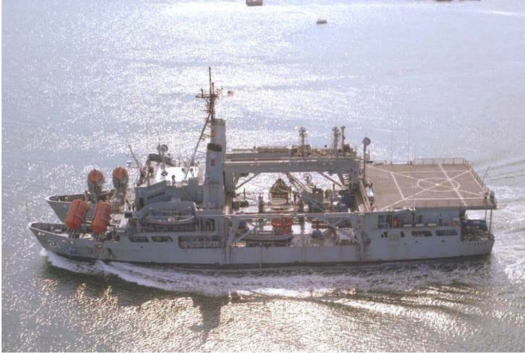
USS Pigeon (ASR-21) underway. Pigeon was the first of two catamaran-hulled SRVs. Location and date are unknown. http://www.navsource.org/archives/09/32/3221.htm
