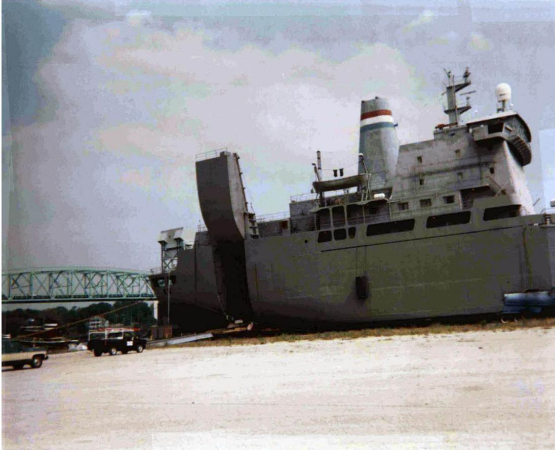
**M/V *Cape Lobos*, starboard quarter view showing after shell cargo door open and vehicle ramp extended. Maritime Administration photograph, date unknown.**
