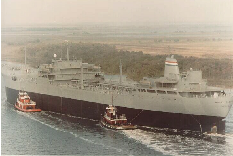
Mount Vernon's sistership, Mount Washington , circa 1980s. Note the divided superstructure, which was typical for tankers when Mount Washington and Mount Vernon Victory were constructed in the early 1960s. Maritime Administration photo.
