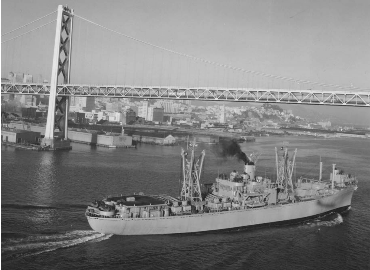
USS Tulare passes under the Oakland Bay Bridge in San Francisco, California, circa 1956. Tulare was the first U.S. attack cargo ship equipped with a helicopter platform. Tulare 's quadrupe masts support the standard contemporary radar systems of the day, the SPS-10 (forward) for surface search and SPS-6 (aft), for air search. Photo courtesy of the Naval History and Heritage Command.
