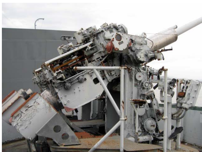
On April 8, 2010, personnel at the Suisun Bay Reserve Fleet removed Tulare's 9-ton twin 3"/50 caliber guns so that they could be installed on the museum/memorial ship USS Hornet (CV-12) located in Alameda. http://www.flickr.com/photos/aheiden/4504047359/
