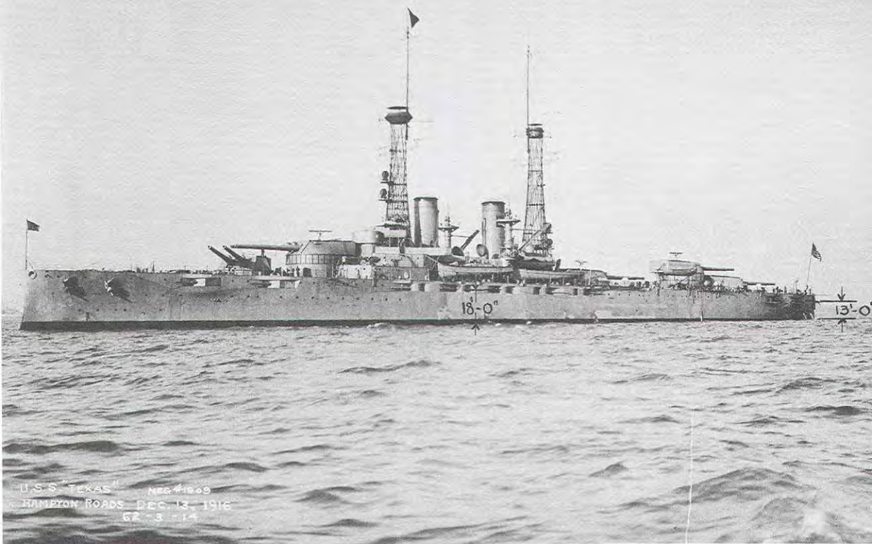
Fig. 24. By December, 1916, when this photograph was taken at Hampton Roads, Texas ' open bridge had received a cover; optical rangefinders were being tried atop turrets 2, 3, and 4; and the radio antennae were becoming more complex. The 3-inch anti-aircraft guns at the tops of the crane kingposts, indicating the beginning of a shift toward a new kind of naval warfare, were the first on any U.S. battleship. Figures inked on the photograph indicate the height above the waterline of the 5-inch guns mounted on the gun deck amidships and astern. Service experience was to prove that those guns were difficult to use in any kind of sea, and all of them were eventually removed. Courtesy U.S. Navy
