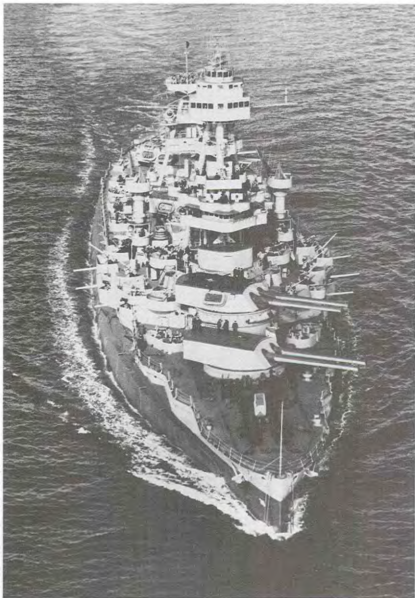
Fig. 12. In 1943 Texas was working with the U.S. Coast Guard as a convoy escort for troopships and transports headed to England in preparation for the invasion of Normandy. The ship's colors at that time were Camouflage Measure 22: gray on the upper hull and vertical surfaces of the superstructure and dark blue on the lower hull and horizontal surfaces, with dark stripes painted along the upper surfaces of the big guns to match them with the dark blue decks. Courtesy National Archives
