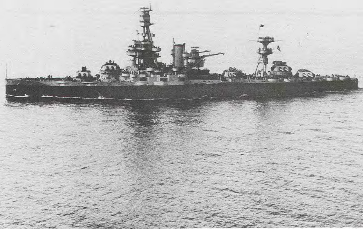
Fig. 28. In 1943 Texas was assigned to escort the huge convoys of transport ships that were supplying the buildup of arms and men for the invasion of France and the assault on German-occupied Europe. Antiaircraft armament at that time included 1.1-inch "Chicago piano" quad mounts. The radar antennae atop the foremost and the after fire control top were for the FC main-battery ranging radar, but an optical rangefinder is still kept in reserve atop No. 4 turret. Courtesy of The Mariners Museum, Newport News, Virginia
