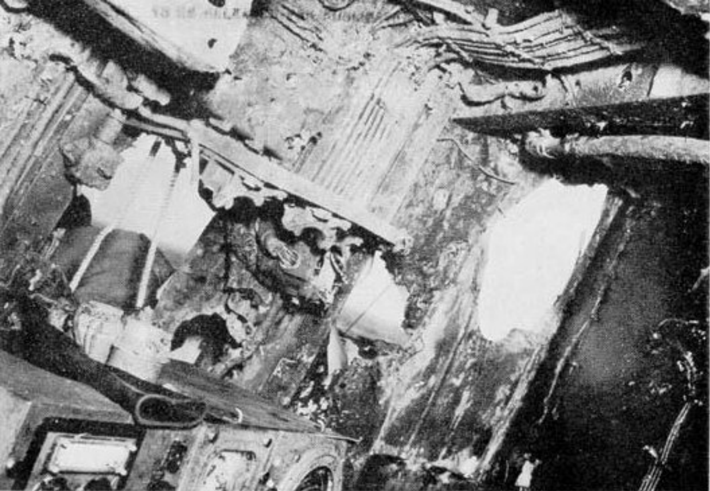
Photo 22: Hits Nos. 13 14 and 15. Damage to port longitudinal structural bulkhead looking from radar plot.
