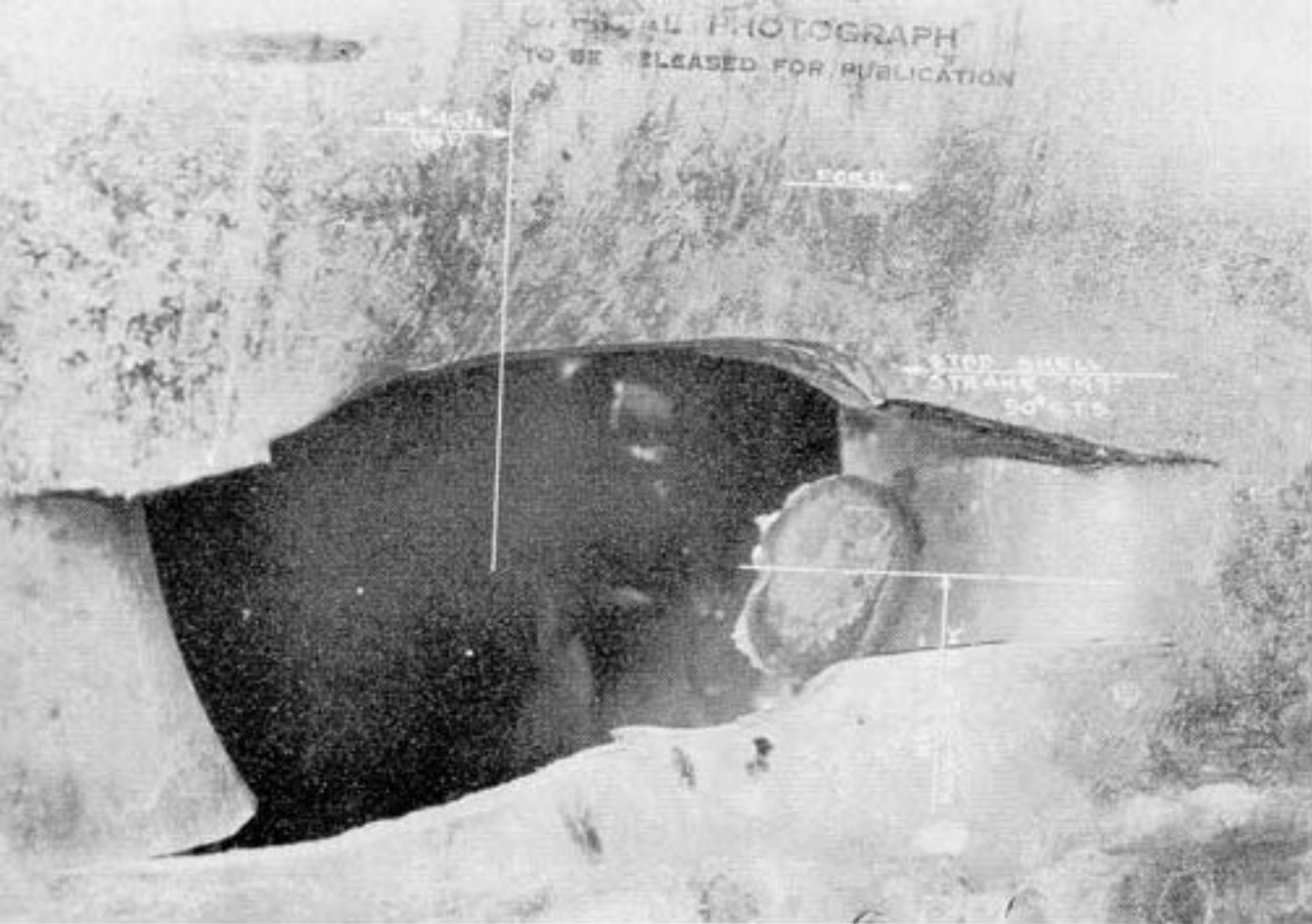
Photo 3: Hit No. 4. Projectile entry hole at frame 46-1/2.
