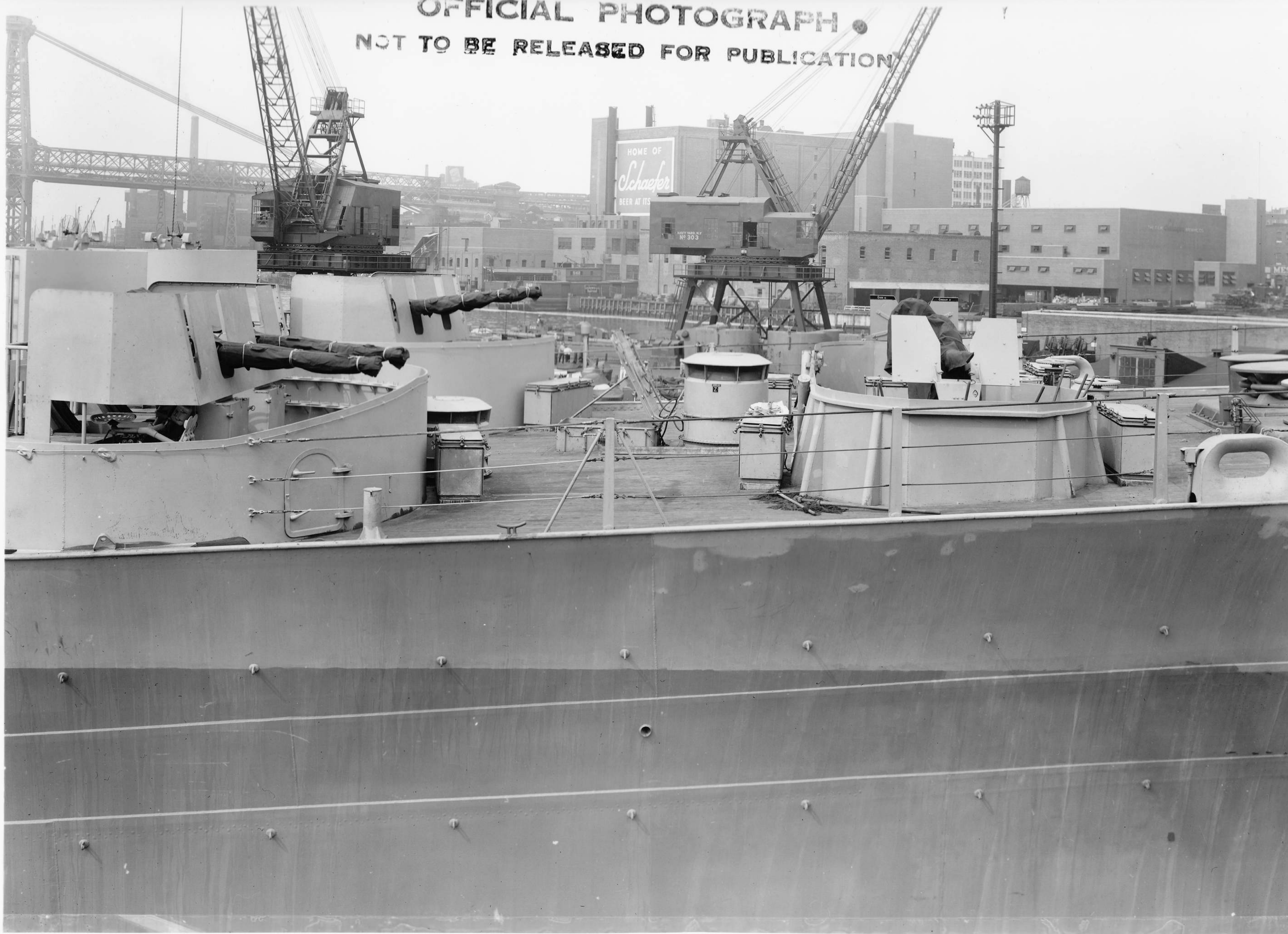
F1111C465 U. S. S. BB 61 40 MM. MTS. MN. DK. FR. 35 & 20 MTS. SIDE VIEW LOOKING TO PORT.
