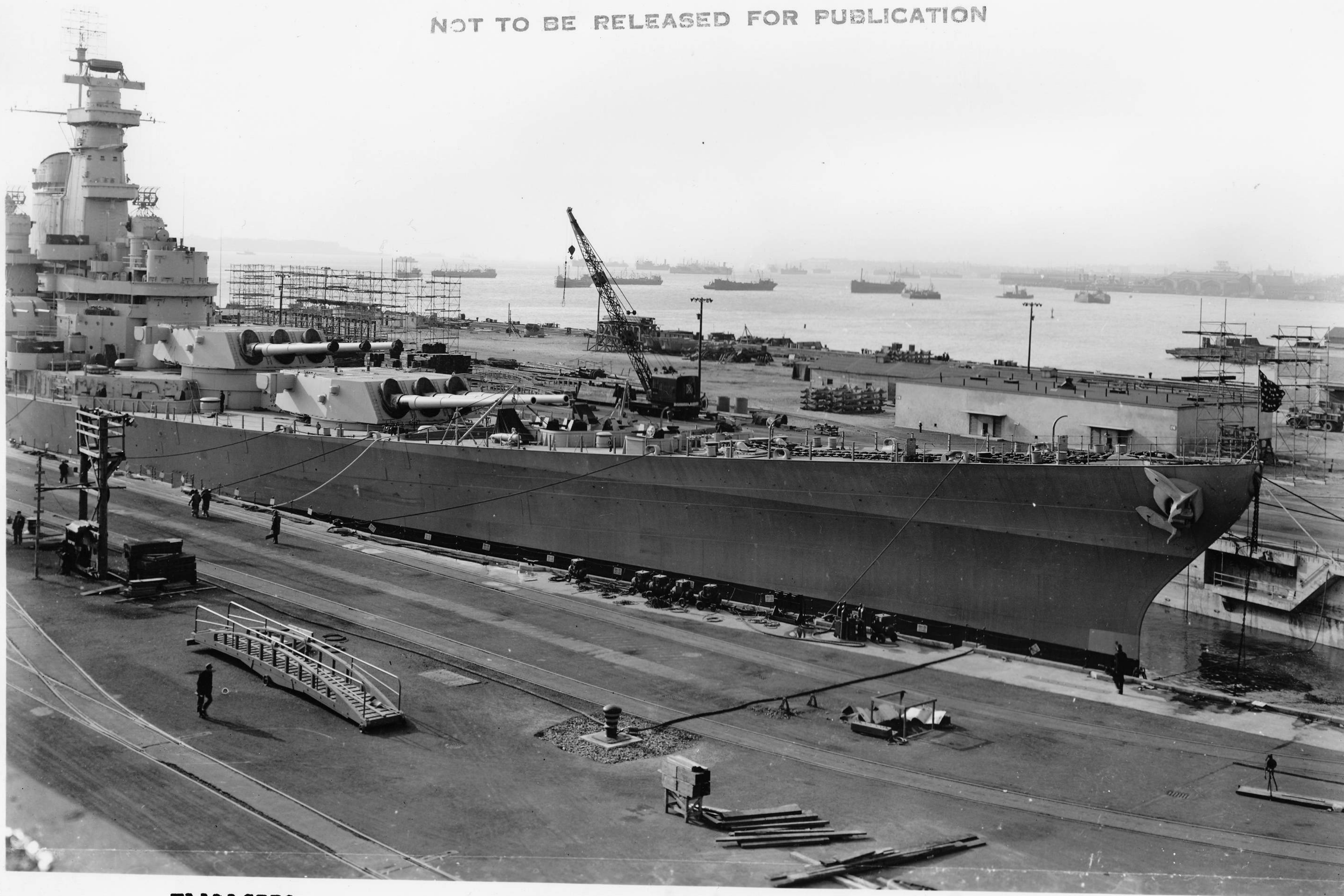
F1111C339 U.S.S. BB 61. INCLINING EXPERIMENT.
