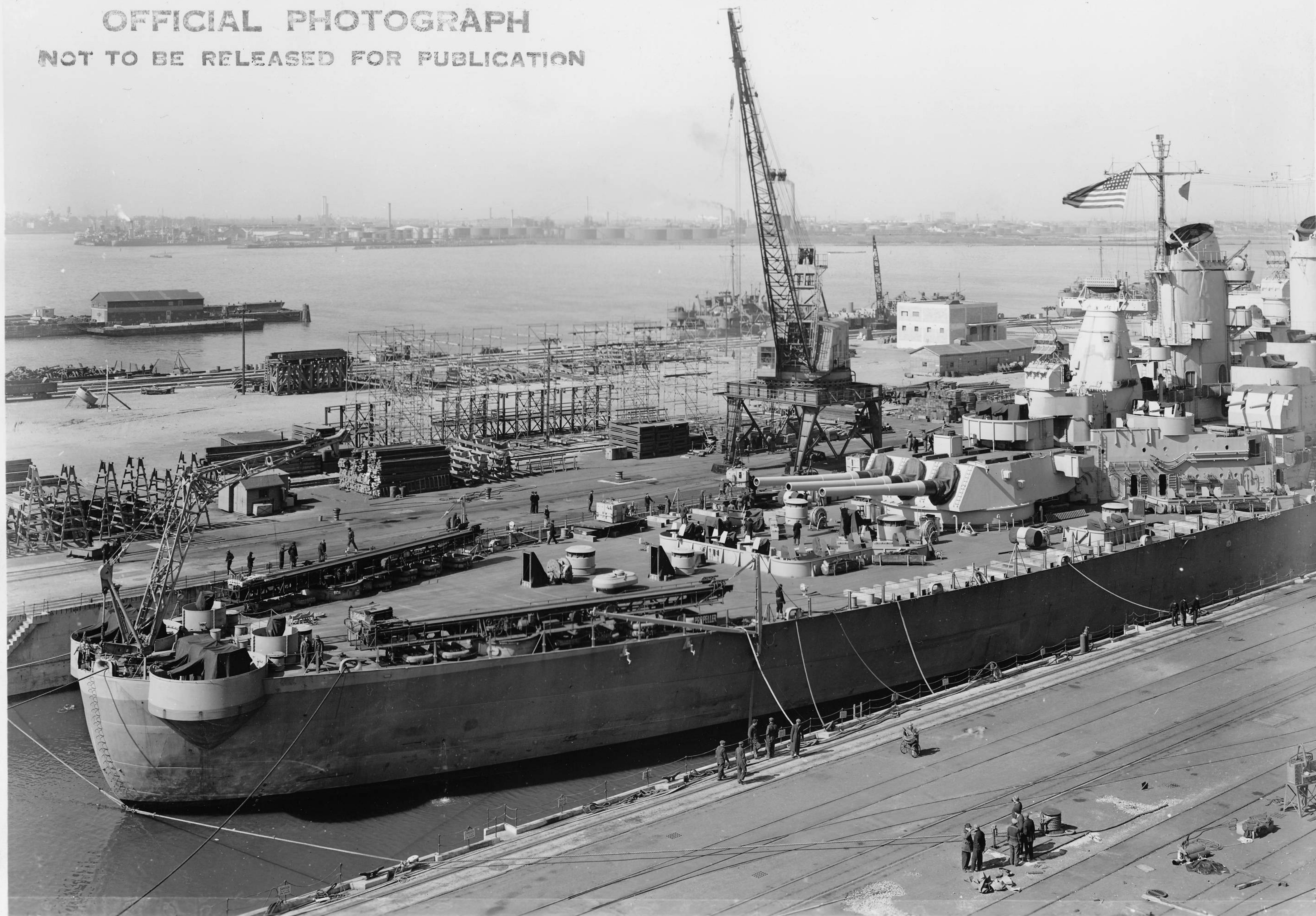
F1111C342 U.S.S. BB 61. INCLINING EXPERIMENT.
