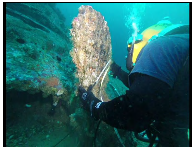
Figure 8: Diver measuring propeller.
