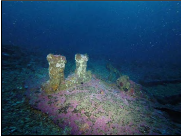
Figure 9: Large double bollard forward of the stern.
