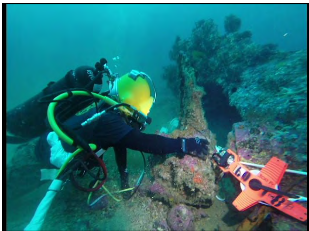
Figure 7: Diver inspects the propeller for any markings and notes missing blade.
