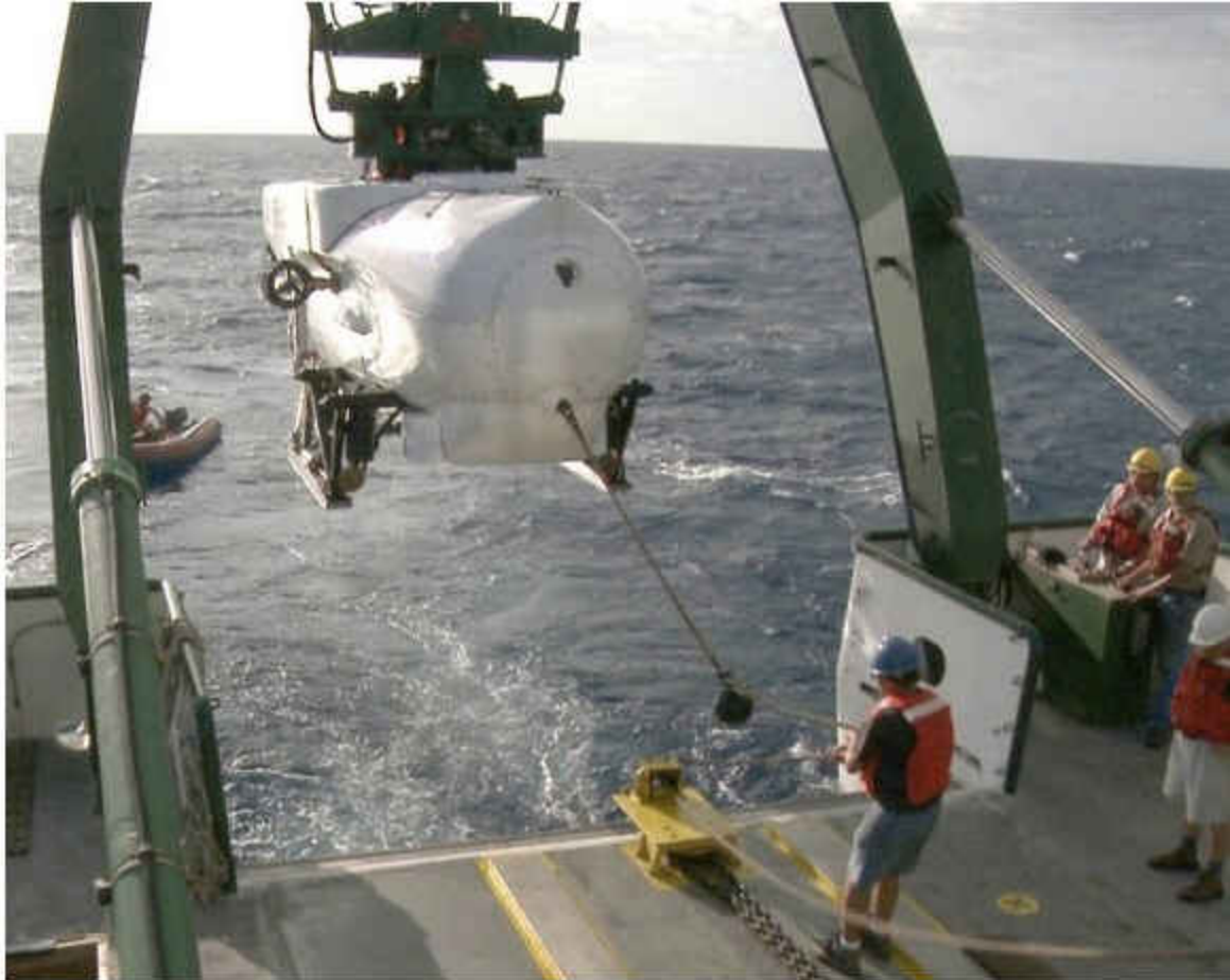
Pisces submersible is recovered from the water onto Ka'imikai-o-Kanaloa ship. The Ka'imikai-o-Kanaloa, also known as the KoK, is the support ship for the Hawaii Undersea Research Laboratory's (HURL's) field operations.
