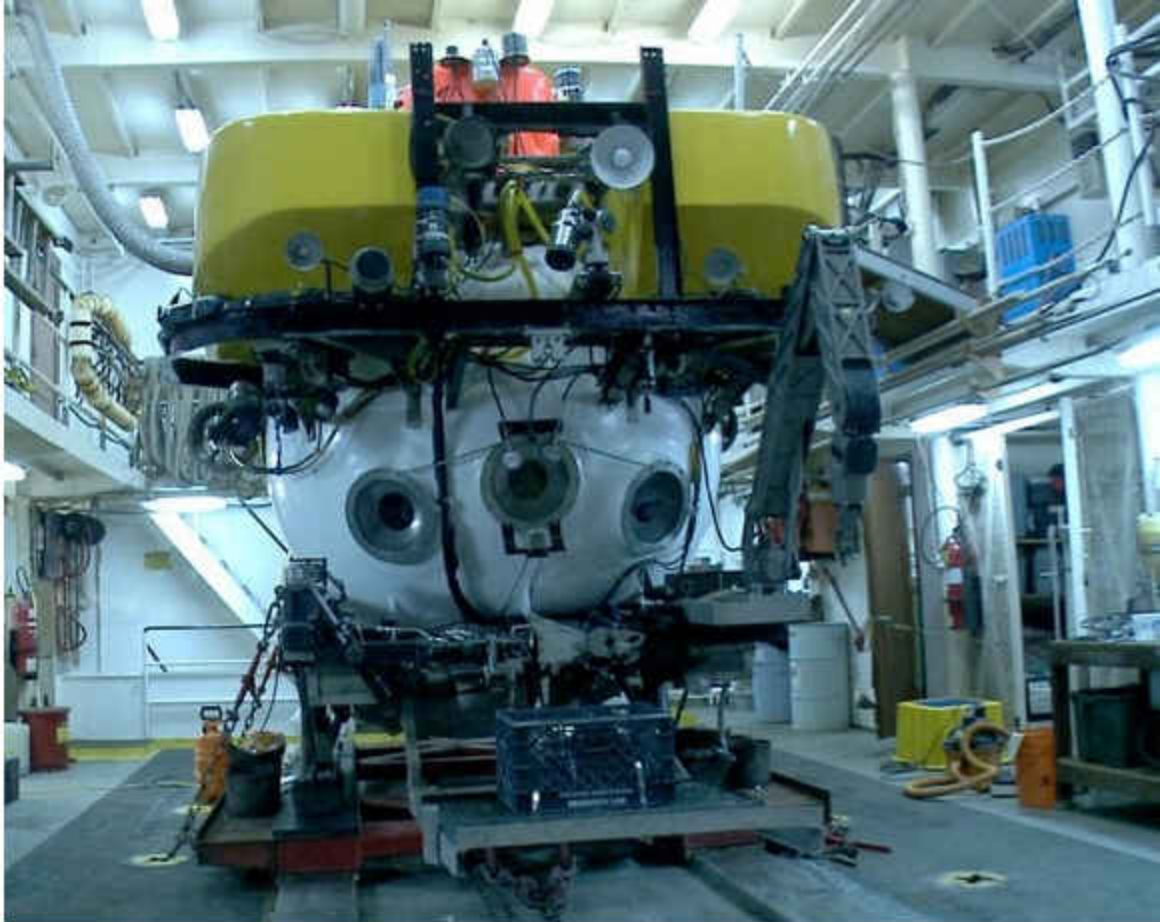
Pisces submersible inside hanger of the Ka'imikai-o-Kanaloa ship. The Ka'imikai-o-Kanaloa, also known as the KoK, is the support ship for the Hawaii Undersea Research Laboratory's field operations.
