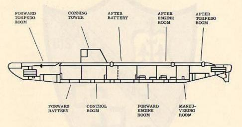
FORWARD TORPEDO ROOM 6 torpedo tubes, torpedo stowage, escape trunk, crew's berthing area
