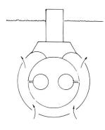
In order to dive, valves at the top of the ballast tanks are opened to vent the air entrapped in those tanks and water floods in through ports at the bottom of the tanks. As the tanks fill, the ship loses positive buoyancy and sinks beneath the surface. Special trimming tanks are used to adjust the ship's weight until it has neutral buoyancy and is balanced fore and aft. Up and down movement is controlled by the diving planes at the bow and stern.
