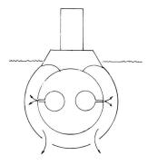
When it is desired to surface, the vent valves at the tank tops are shut and compressed air from storage bottles is released into the tanks. The expanding air expels the water out the flood ports, until the tanks are empty once more and the submarine floats to the surface.
