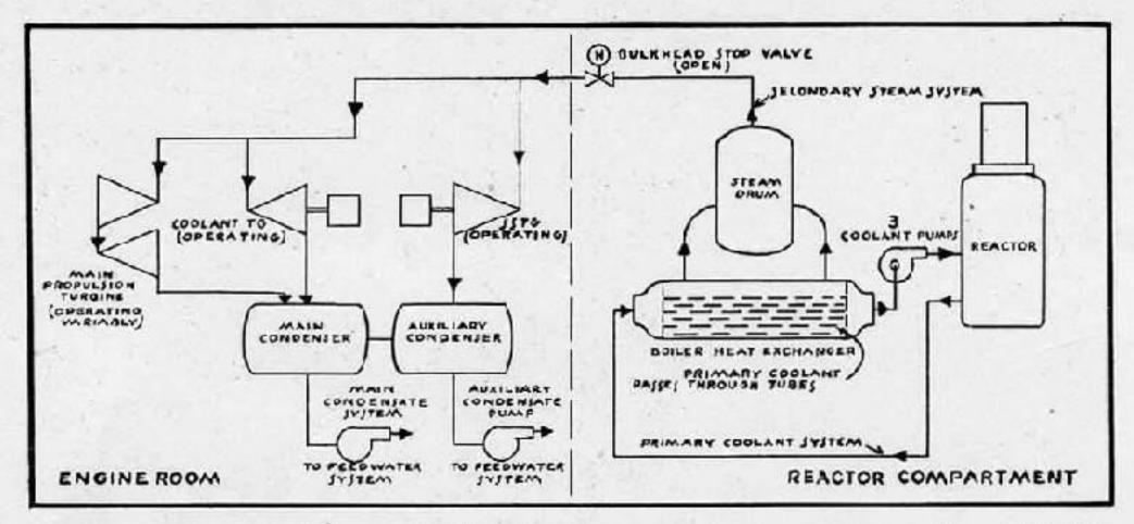
while the secondary water which is boiling to make steam is on the shell side of the boiler.
