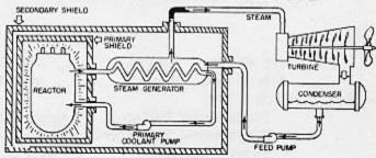
THRESHER is powered by a nuclear power plant which consists of a nuclear reactor with its associated circulating water and steam cycles and auxiliary machinery.
