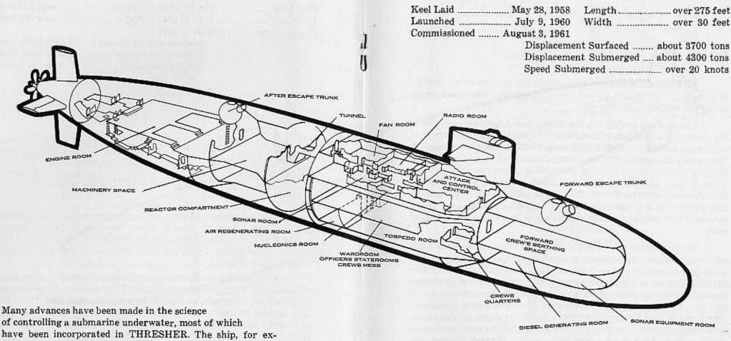
Many advances have been made in the science of controlling a submarine underwater, most of which have been incorporated in THRESHER. The ship, for example, can be controlled both on course and in depth by a single man. An automatic feature is also included in the control system which keeps the ship at the ordered depth.
