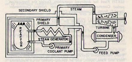
The power plant of a nuclear submarine is based upon a nuclear reactor which provides heat for the generation of steam. This, in turn, drives the main propulsion turbines and the ship's turbogenerators for electric power.
