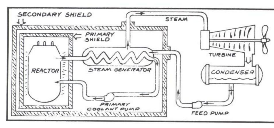
JAMES MONROE is powered by a nuclear power plant which consists of a nuclear reactor with its associated circulating water and steam cycles and auxiliary machinery.
