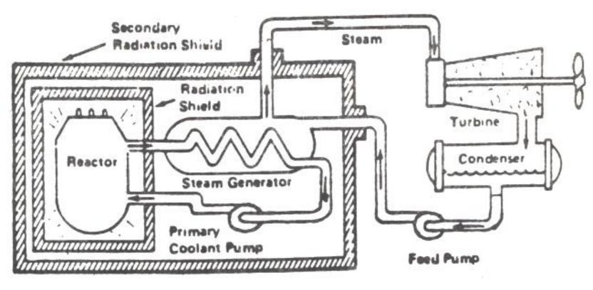
THERE IS NO STEP IN THE GENERATION OF THIS POWER WHICH REQUIRES THE PRESENCE OF AIR/OR OXYGEN. THIS ALLOWS THE SHIP TO OPERATE COMPLETELY INDEPENDENT FROM THE EARTH'S ATMOSPHERE POR EXTENDED PERIODS OF TIME.
