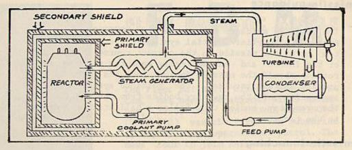
JAMES MONROE is powered by a nuclear power plant which consists of a nuclear reactor with its associated circulating water and steam cycles and auxiliary machinery.
