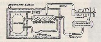
THE WOODROW WILSON is powered by a nuclear power plant which consists of a nuclear reactor with its associated circulating
