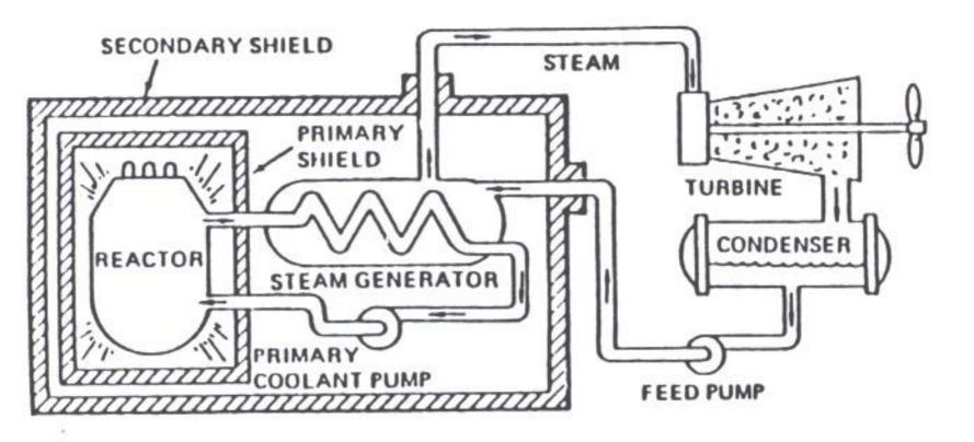
The power plant of a nuclear submarine is based upon a nuclear reactor which provides heat for the generation of steam. This, in turn, drives the main propulsion turbines and the ship's turbo-generators for electric power.
