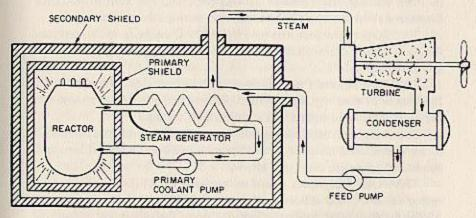
In the steam generator, the heat of the pressurized water is transferred to a secondary system to boil water into steam. This secondary
