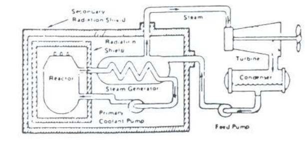
The propulsion plant of a nuclear powered ship is based upon use of a nuclear reactor to provide heat. The heat comes from the fissioning of nuclear fuel contained within the reactor. Since the fissioning process also produces radiation, shields are placed around the reactor so that the crew is protected.
