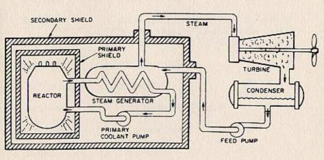
In the steam generator, the heat of the pressurized water is transferred to a secondary system to boil water into steam. This secondary system is isolated from the primary system.
