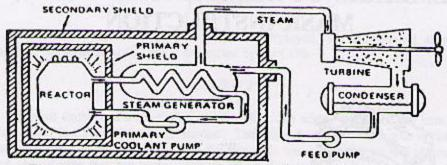
The power plant of a nuclear submarine is based upon a nuclear reactor which provides heat for the generation of steam. This, in turn, drives the main propulsion turbines and the ship's turbine generators for electrical power.
