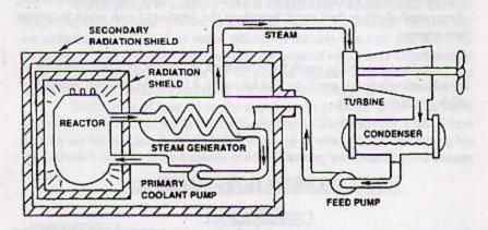
Note that no part of the generation of power from a nuclear submarine requires the presence of air or oxygen. This allows the ship to operate completely independent from the earth's atmosphere for extended periods of time.
