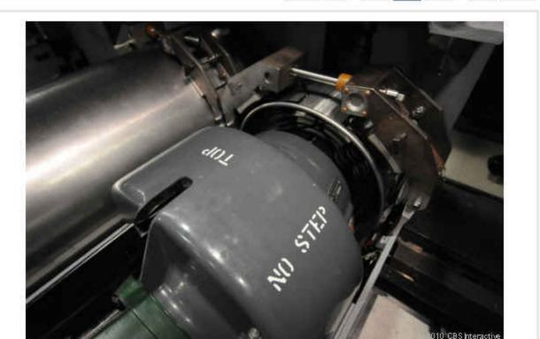
At the end of the Mark 48 torpedo, this extra device spools out up to 25,000 yards of fiber-thin cable. By staying connected to the submarine, the torpedo can keep constant communications with firing control, which can update the target profile in real time. If the fiber is broken, the torpedo still has enough information and autonomy to complete its last understanding of the target's location and trajectory.
