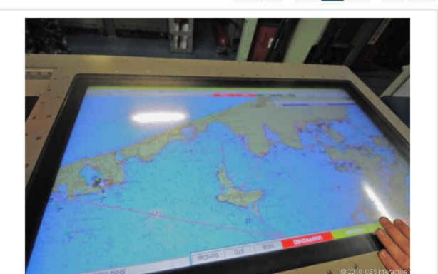
This digital screen shows the North Carolina's coordinates, or any other location, either by virtue of GPS when above water, or if under water, by a sophisticated system of sensors that keep highly accurate track of the boat's movement in three dimensions.
