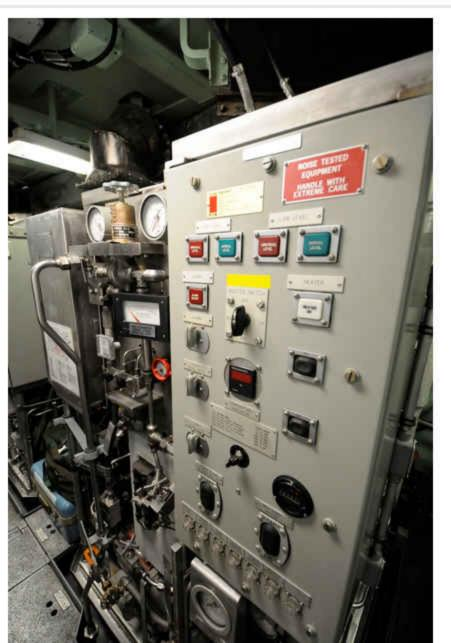
After going through the carbon monoxide burner, the resulting carbon dioxide is removed by this scrubbing machine. There are two of these for redundancy's sake.
