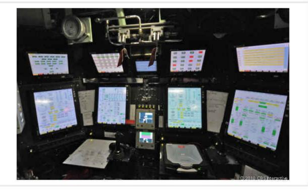
In the past, submarines had one sonar room, where the commander could look out through the periscope and where the sonar work was done; and a second room for the drivers of the sub. Now, thanks to modern communications, navigation and driving systems, those separate rooms have been combined into one, modern nerve center.
