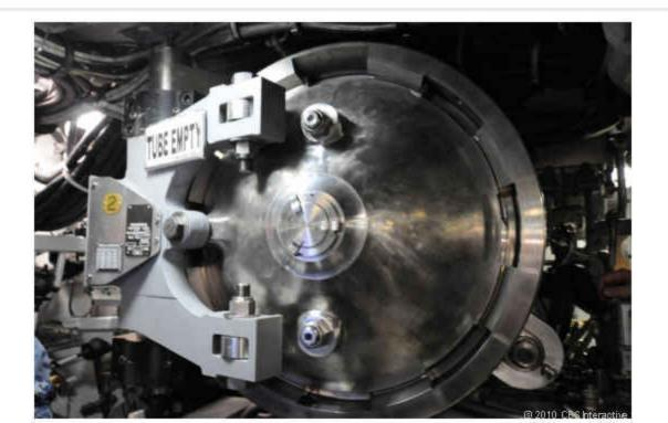
Using the special cradle system, the torpedoes are moved into place and then are essentially shoved at high speed out of these tubes. It takes a highly efficient crew about 10 to 15 minutes to prepare and launch a torpedo, though a crew can be working on launching multiple torpedoes in succession.
