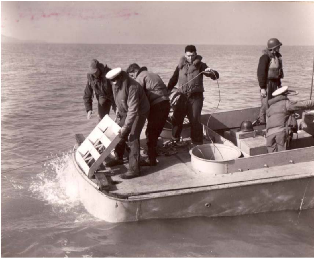
Streaming moored minesweeping gear from an LCVP – Chinnampo, North Korea Oct 1950
